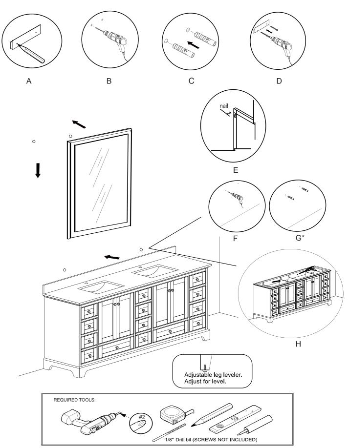
\*SECURE SCREW TO STUDS WHEN POSSIBLE
