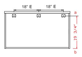
Step 1: Metal plates has been pre-installed to the back of cabinet, measure the distance between the bottom of the cabinet and point a.
