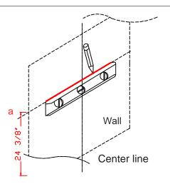
Step 2: Draw a horizontal line from the point a by using a leveler. (suggested H24 3/8" from floor to "a" line)
