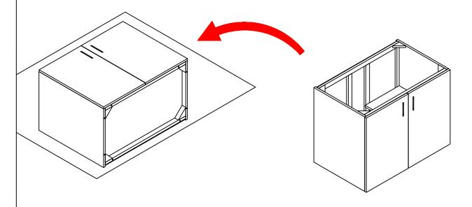
Step 1: To attach the metal legs, place the cabinet lay down on a blanket or similar soft material.
