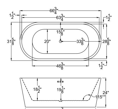
$\begin{array}{c} 3267V \\ 31\frac{5}{8} \text{" x } 66\frac{3}{4} \text{" x } 24 \text{"} \end{array}$
