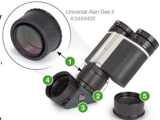
The Universal Alan Gee II ① is connected with the help of the included 7,5mm extension ring ② onto the T-2 star diagonal ③. The star diagonal is attached to the telescope either through the BTA-adapter for Schmidt-Cassegrains #2408160 ④ or a 2"/T-2 nose piece #2408150 ⑤.
