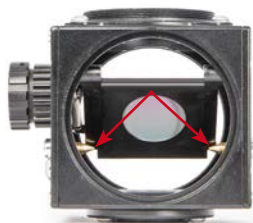
The two pins on which the mirror lays on
