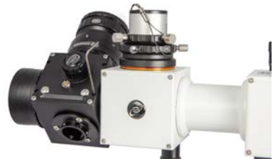
The orientation of the adapter threads on both sides can be changed with the four grub screws. This way, you can align instruments like the DADOS spectrograph in this image to the BFM II, or you can rotate the whole BFM, if it is screwed directly to the telescope.
