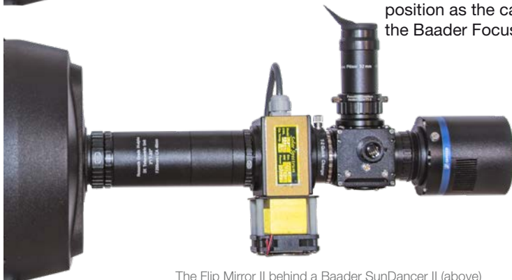
The Flip Mirror II behind a Baader SunDancer II (above) and a SolarSpectrum Filter (below, without the additional 40 mm T-2-extensions).
