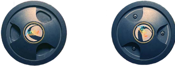
The collimation screws in the secondary mirror mount. On the TriBand C8 they are exposed, on the TriBand C9¼ and C11 they are under a cover flap (left), which you have to turn to expose the screws (right).
