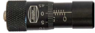
The micrometer screw can tilt the filter to easily observe the blue wing of the H-alpha-line
