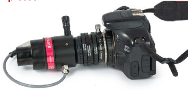
A DSLR with 0,4x telecompressor and T-2 quick-changer
