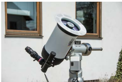
The SunDancer II at a 8" Triband SC where the D-ERF is part of the Schmidt corrector plate.
