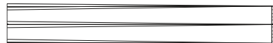
Light beam of a 6" lens telescope, which was extended to f/30 with a telecentric system
