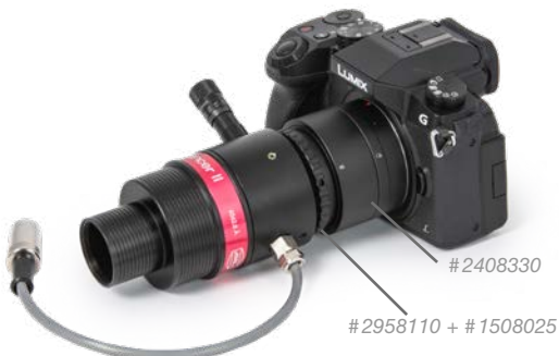
A DSLR with a standard T-ring still needs a 10mm T-2 extension. A standard T-ring has an overall length of 55 mm - here using the example of a mirrorless Micro Fourthirds camera with the Micro Fourthirds T-ring #2408330 (with 19 mm extension).
