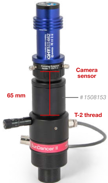
A planetary camera with 1¼" plug-in sleeve. A 40 mm T-2 extension sleeve provides the ideal working distance of 65 mm.
