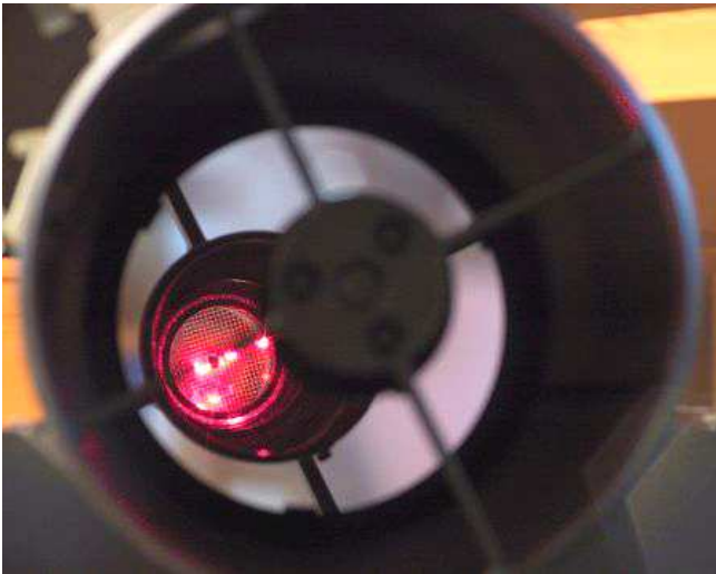
Picture above again shows the view from the tube's front to the reflected images of the secondary mirror and the grid plane.
