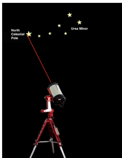
Figure 4.4b. Alt-Az mode Polar Alignment
