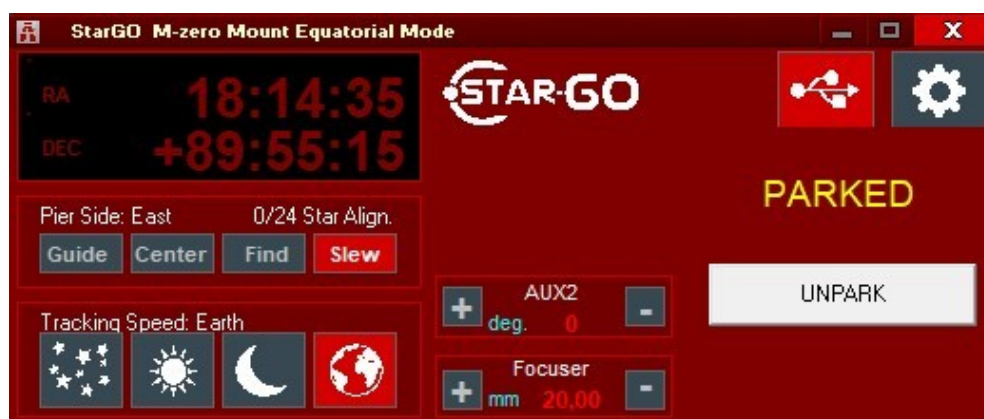
Figure 3.1.b Main Panel with the mount parked
