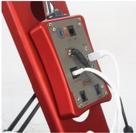
Figure 1.3b: StarGO power connection
