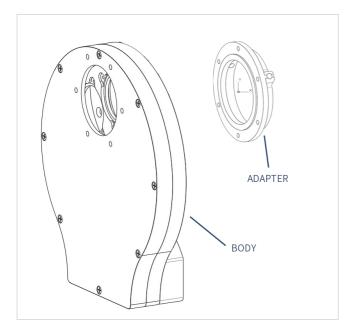
We list BFL consumed data of both CFW body and adapter at our Adapter System 2.0 instructions (like kit A1, see below). When you use some kits of Adapter System 2.0, you may need to remove this filter wheel adapter. (like kit A2, see below).
