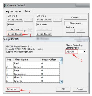
A new ASCOM Filterwheel Chooser window pops up. Select the connected filter wheel in the strip box. Click on Properties to determine the filter wheel properties. Make sure to select the port that matches the previous download driver, click ok to return to the Camera Control page.
