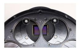
We recommend you only fix these four screws when the cam is not heavy, like 294M and 268M. That is firm enough and no need to remove the filter holder when you want to seperate them.
