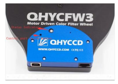
Use the USB cable to plug into the USB port of the filter wheel and the other end to connect to the computer.
