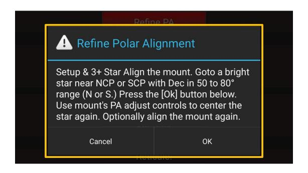
Make the bright star move to the center of your field of view by manually adjusting the mount's azimuth and altitude angle.
