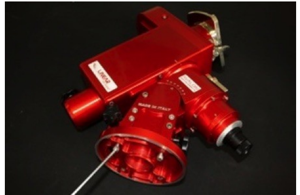
2) Unscrew the 4 screws of the side bracket
