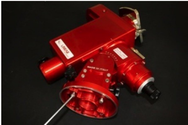
1) Unscrew the 2 screws under the base
