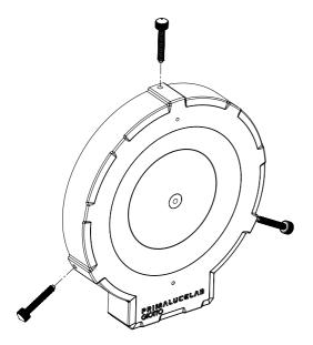
GIOTTO smart flat field generator includes thumbscrews to allow you to affix it to front of your telescope, letting you easily record flat calibration files for astrophotography. A range of GIOTTO models are available, allowing you to calibrate telescopes of different diameters. In the box you will find 3 thumbscrews (made of plastic so they won't mark your telescope). Insert the 3 thumbscrews into the M6 threaded holes of GIOTTO approximately halfway.
