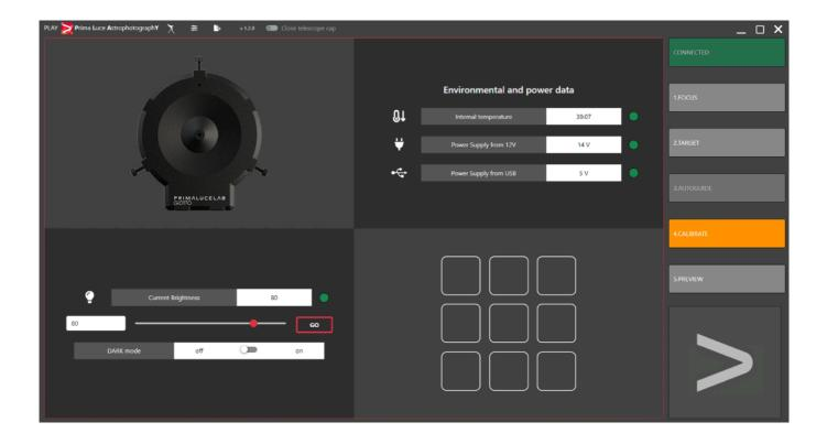
7) To illuminate GIOTTO, select a brightness level with the slider and change the switch from OFF to ON. This will turn on the flat panel light at the desired intensity.
