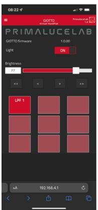
The Virtual HandPad allows you to save up to 9 preset brightness values for your GIOTTO. In order to save a brightness value in the Virtual HandPad, tap and hold one of the empty buttons: the position will be automatically saved with a "Preset" name.
