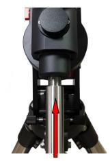
5. Install Counterweight(s): Before putting on CW, make sure the mount is at its zero position, i.e., CW shaft points to the ground. Disengage the R.A. Gear Switch to set the R.A. axis free before loading the CW. Remove the CW Safety Cap at the end of CW Shaft. Glide the CW over the shaft. Tighten the CW Locking Screw to hold the CW in place. Place the Safety Cap back onto the shaft. Move the CW to the bottom of the shaft and tighten the CW locking Screw.
