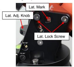
Two latitude ranges, 14~44° and 36~68°, can be set up for the mount head. To change the latitude range from one to the other, **both** the Latitude Position Bolt and the Latitude Locking Screws need to be moved to the correct locations (see photos below).
