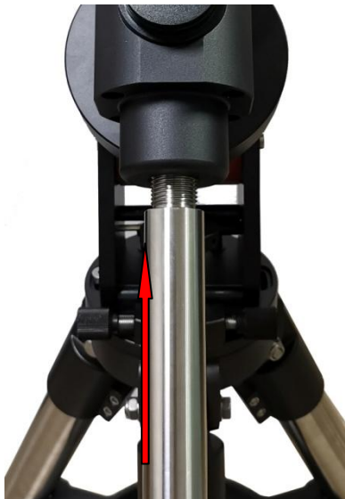
Figure 16. Install CW shaft
