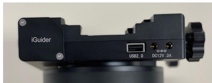
Figure 4. Port on back of the dovetail saddle (a GEM45G shown)
