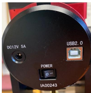
Figure 2. GEM45 Power Panel on Rear of RA axis
