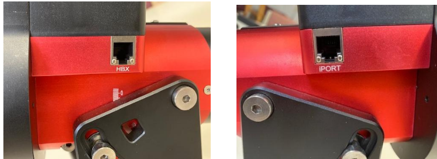
Figure 3. Ports on a GEM45 main board
