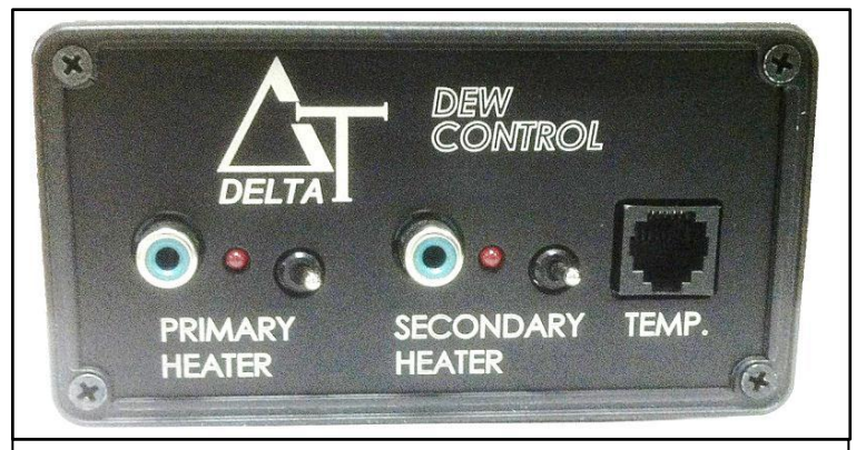
Fig 4 – Rear electronics panel on the Delta-T controller
