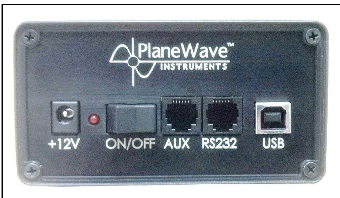
Fig 3 – Front electronics panel on the Delta-T controller
