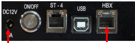
CEM70 Power and HC connection
