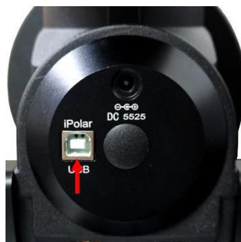
Figure 24. Connect CEM70/EC iPolar to a computer
