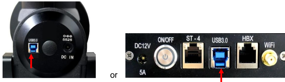
Figure 23. Connect CEM70G iPolar to a computer
