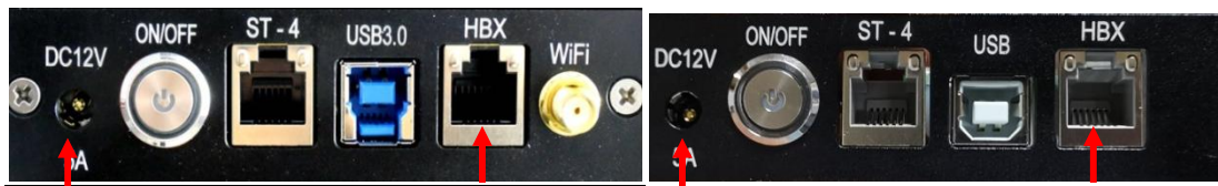
Figure 22. CEM70G (left) and CEM70/EC (right) mount base panel
