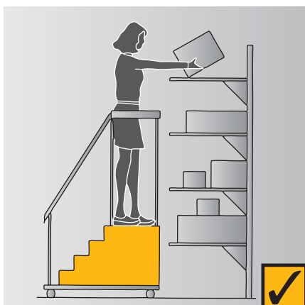
Figure 4.18 Controlling risk of storage at height
