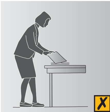
Figure 4.8 Incorrect standing-height bench
