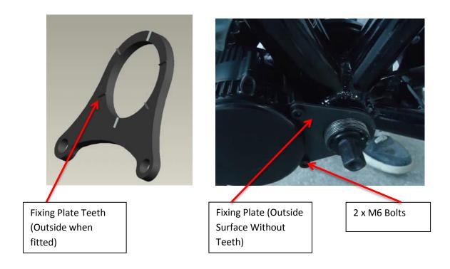
5. Hold the drive unit up against the frame and tighten the M6 x 10mm bolts and M33 nut simultaneously. Tighten M33 with force 30-40Nm. If you purchased an installation toolkit use the BBB Lockring tool.
