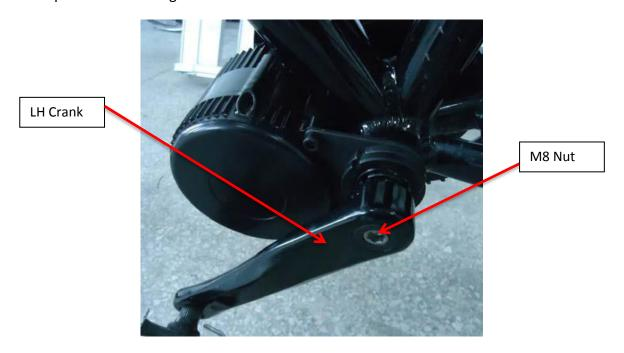
8. Fix the RH crank on the bike with the M8 inner hex bolt. Tightening force 35-40Nm. Use Loctite if you wish as this bolt is prone to loosening.
