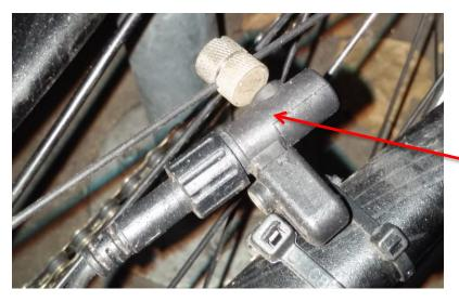
Speed Sensor – Optimal position of magnet is less than 5mm from Sensor on rear wheel.
