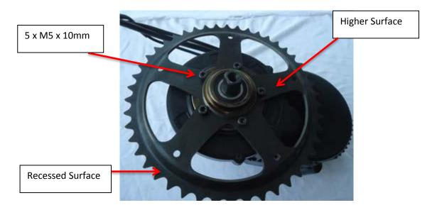
3. Carefully feed the drive unit axle through the bottom bracket. If you encounter resistance your BB shell may need to have burs / weld overflow smoothed with a rounded file.
