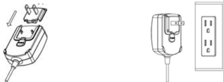
Figure 2-4. Connecting the AC adapter to AC supply
