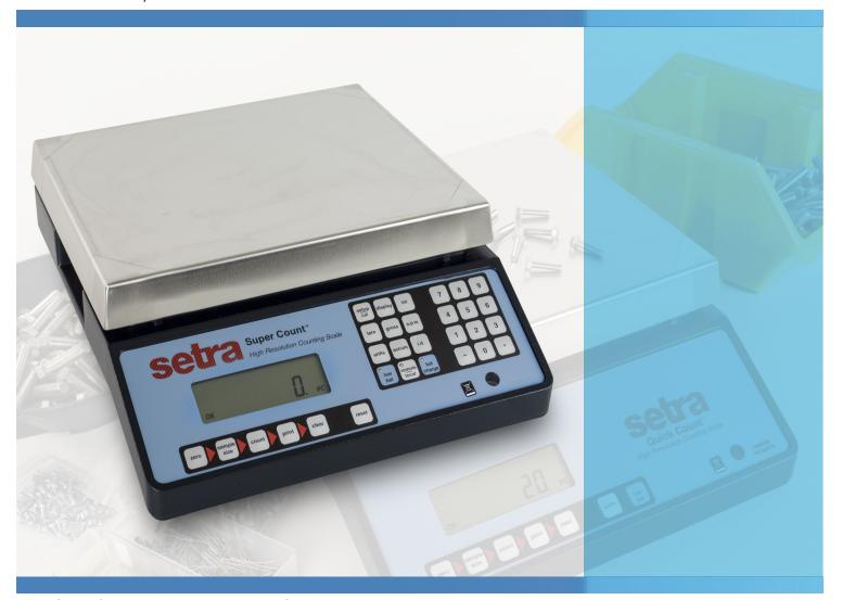
The Super Count couples the benefits of Setra's high resolution ceramic sensor with an intelligently designed, full-function keyboard to deliver a high accuracy, easy-to-use counting scale at a surprisingly moderate price.
