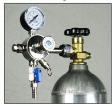
Attach 5/16" I.D. tubing to regulator nipple and clamp into place. Make the tubing more pliable by heating the end up in boiling water.
