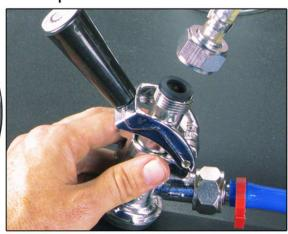
Home Brew Couplers - Home brew couplers have a separate attachment for the gas in and liquid out. The air tube attaches in the same manner as the commercial coupler. The liquid out home brew coupler uses a hose nipple so you must cut off the fitting on the end of the beer line to attach it to the liquid out coupler. Clamp each hose into place.
