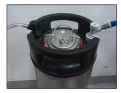
If you will be switching back and forth from home brew to commercial kegs, it is a good idea to keep the fittings from the end of the beer line and attach them to the top of your commercial keg coupler. Then you will have a 3/16" hose nipple on top of each coupler, allowing you to unclamp the hose from one and attach it to the other.
