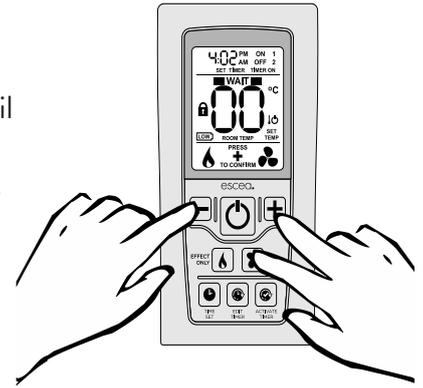
3. Press and hold the – (minus) button until the two large temperature digits reading 00 start to flash slowly. Release the – (minus) button. The remote control is now ready to be addressed to the fire.
