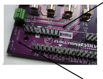
• If you have Allteksystems LED/Lamp Driver or the Aux LED/Lamp Driver, you can also attach the LED wire directly from the board to one of the 2 lugs in the corner of the new rectifier board.
