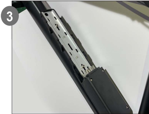
After taking out battery.
