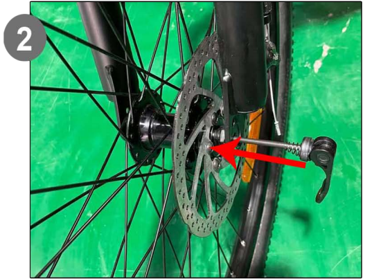
The front fork is aligned to both ends of the bearing. The disc brake is on the left.
