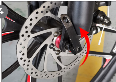
Twist the wrench upward and check the operation of the wheel
