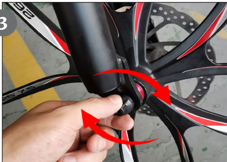
Install the quick release and nut then tighten well
