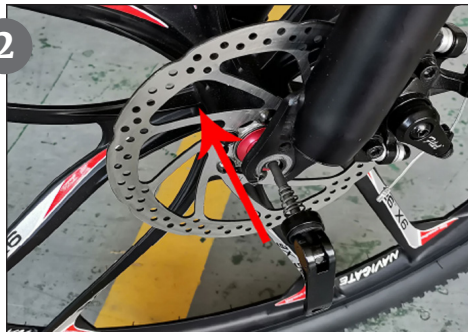
The front fork is aligned to both ends of the bearing. The disc brake is on the left
