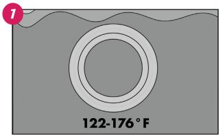
**STEP 1:** Soak tire in hot water for 5-10 minutes to make it softer and easier to install. Immerse tire completely.
