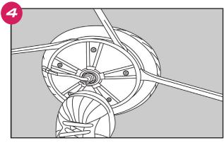
STEP 4: Hold the tire secure with your foot, use a tire lever to press the whole tire onto the rim.
