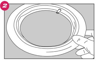
STEP 2: When the tire is soft enough, insert the inner tube into the tire.
