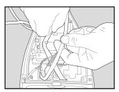
**STEP 6:** The battery has cables clipped so that wires are not loose in the hoverboard. Unhook the cables from the clip on the battery.
