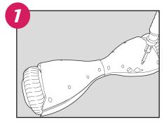
**STEP 1:** Flip over the hoverboard and unscrew all 8 screws (be sure to keep them in a safe place)
