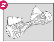
**STEP 2:** Carefully lay the covers down being careful to not remove the wires from the cover.
