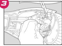
**STEP 3:** Unplug the cable with the yellow cap. (this is the side of the board that has the cable connected to the cap)
