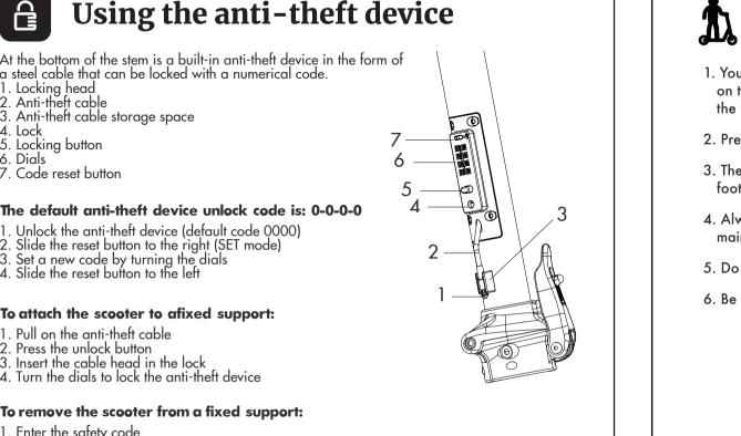
the cable head in the storage bracket to prevent it from hanging down and
