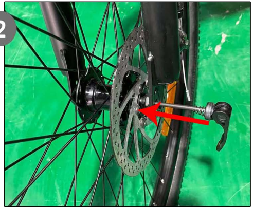
The front fork is aligned to both ends of the bearing. The disc brake is on the left.
