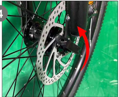
Twist the wrench upward and check the operation of the wheel.
