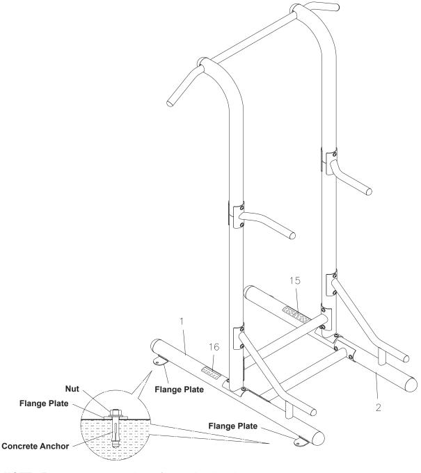
NOTE: Four concrete anchors (mounting hardware not included) are needed to secure the LEFT and RIGHT BASES(1, 2) of the STAMINA® Outdoor Power Tower, two on each side.
