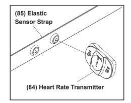
To wear the **HEART RATE TRANSMITTER(84)** around the chest, hook the hook end of the **ELASTIC SENSOR STRAP(85)** to the other end of the **ELASTIC SENSOR STRAP(85)**. Adjust the **ELASTIC SENSOR STRAP(85)** to fit your chest snugly as shown in the illustration below. Apply water or conductive gel to moisten the heart rate sensor electrodes. These heart rate sensor electrodes must be wet and in contact with your chest skin to properly detect your heart rate.
