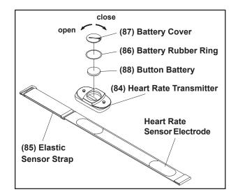
Refer to the illustration. Press the **HEART RATE TRANSMITTER(84)** onto the buttons on the **ELASTIC SENSOR STRAP(85)**.
