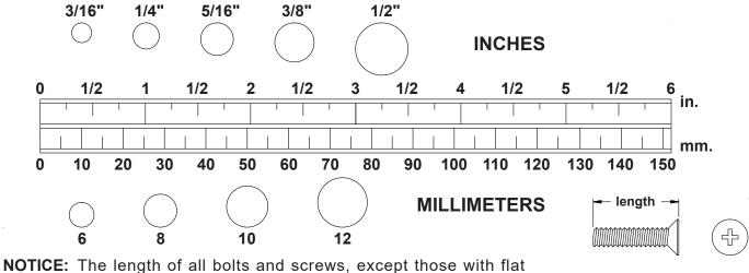
heads, is measured from below the head to the end of the bolt or screw. Flat head bolts and screws are measured from the top of the head to the end of the bolt or screw.
