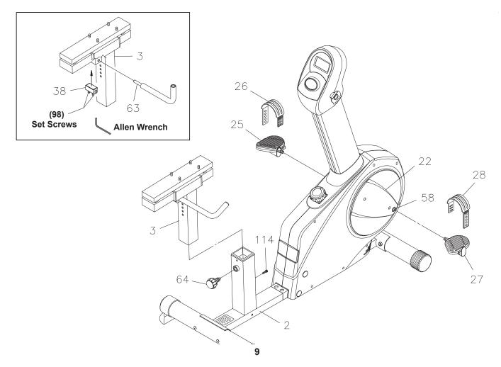
**NOTE:** Be careful not to damage the **PULSE SENSOR WIRES(104)** while doing assembly Step 8 and Step 9.
