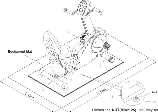
Loosen the **NUT(M8x1.25)** until they touch the **LEVELING STAND(65)**. Adjust the **LEVELING STAND(65)** for leveling. Tighten the **NUT (M8x1.25)** securely against the **REAR FRAME(2)** to lock the stand in position.
