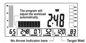
When running the target watt control program, the program will monitor your pedaling speed and adjust the workload automatically to keep your workload as close as possible to the preset target WATT. For example, if the preset target WATT is 120 and you pedal with proper speed, the display will be as shown in the illustration. There should be no Arrow Indicator appearing on the display.
