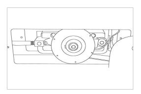
2. Using a long tool, push out the rear end cap as pictured below left. This will give you access to the Tank tensioning Bolt (shown lower right).
