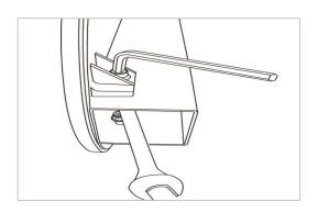
4. Using a 6mm Allen Key, tighten the Belt using the Tank Tensioning Bolt until the belt no longer slips during hard rowing.
