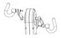
NOTE: Handle threads have a blue coating which will feel very tight when threaded onto crank arm. This is a type of thread locker, which once in contact with the crank arm will cause threads to activate. Note: Allow 15 minutes for the thread locker to activate before first time use. Check pedal tightness periodically thereafter with a 15mm wrench. DO NOT USE IF NOT TIGHT.
