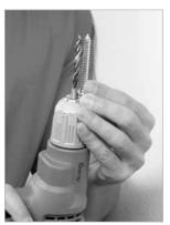
**3. Drill Bit.** Using a standard ½-inch drill bit, measure the drill bit against the length of the lag screw. The drill bit in the photo happens to be the same length of the lag screw (about 2½-inches).
