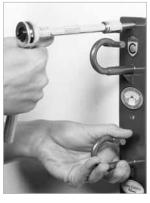
7. **Socket Wrench.** Tighten the lag screw with the socket wrench.
