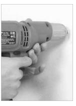
5. **Drill Bit & Lag Screw.** It is important to use a 1/4-inch drill bit. Since the lag screw's diameter is 5/16-inches, the threads of the lag screw will firmly grip the wood stud.
