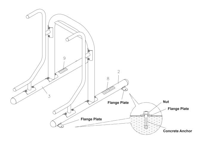
NOTE: Four concrete anchors (mounting hardware not included) are needed to secure the LEFT and RIGHT BASES(2, 3) of the STAMINA® Outdoor Multi-Station, two on each side.
