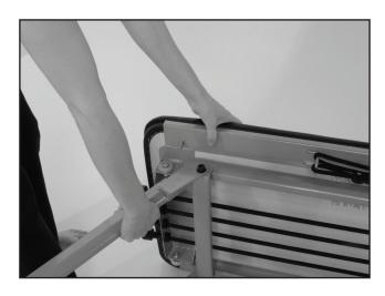
Turn the platform upside down so it is cord side up. Using a crescent wrench and flat head screwdriver, remove the screw that is holding the roller in place. Replace the old roller with the new one, add the washer, push the screw through the roller and tighten with the nut. Do not overtighten the nut. Roller must turn freely.
