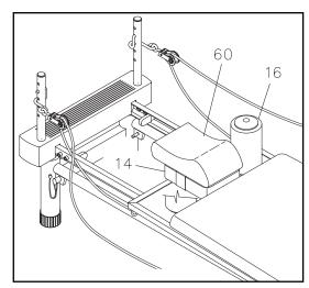
Make sure that both FOAM PADS(16) are in the platform when using the HEADPAD(60) attached to the HEADREST(14).
