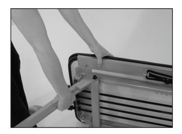
Turn the platform upside down so it is cord side up. Using a crescent wrench and flat head screwdriver, remove the screw that is holding the roller in place. Replace the old roller with the new one, add the washer, push the screw through the roller and tighten with the nut.
