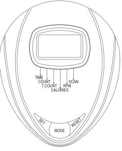
**RESET :** In the **STOP** mode, press the button to reset the setting values to zero. Press the button and hold it down for three seconds to reset all functions to zero.
