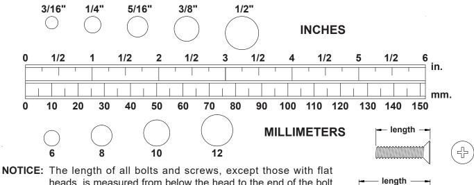
heads, is measured from below the head to the end of the bolt or screw. Flat head bolts and screws are measured from the top of the head to the end of the bolt or screw.
