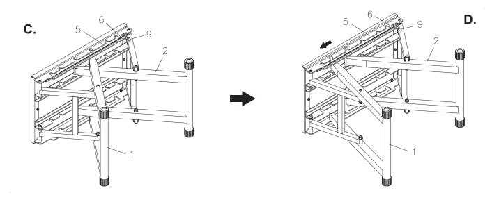
Then adjust the INNER LEG(2) as shown in illustration E. Lock the OUTER LEG(1) and INNER LEG(2) in position with the SAFETY BAR(6), properly secure the SAFETY BAR(6) with the SPRING PIN(9). Place the STAMINA X-Adjustable Plyo Box in the upright position.
