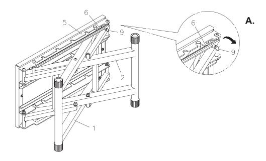
STEP 2: Adjust the height by sliding the OUTER LEG(1) and INNER LEG(2) to the desired positions. Pull the SPRING PIN(9) and flip the SAFETY BAR(6) to lock the OUTER LEG(1) and INNER LEG(2) in position, then release the SPRING PIN(9) to secure the SAFETY BAR(6) properly. Refer to detail view B. Place the STAMINA X-Adjustable Plyo Box in the upright position.
