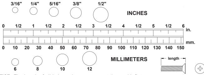
NOTICE: The length of all bolts and screws, except those with flat heads, is measured from below the head to the end of the bolt or screw. Flat head bolts and screws are measured from the top of the head to the end of the bolt or screw.
