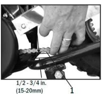
2. If after step. 1 tightening the nut of chain adjustor the chain is still too loose or too tight, <u>another nut at the underpart</u> <u>of chain adjustor</u> must be adjusted accordingly.
