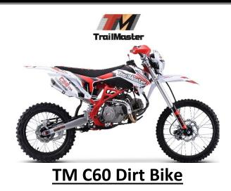
The TM C60 is a great mid size dirt bike. It has a high performance 156cc 4 stroke 14hp engine with kick start and a top speed of around 55 MPH and a seat height of 34.6". It is available in red, green, and orange colors. The TM C60 features a 4 speed manual transmission with front and rear disc brakes, and inverted front shocks! This is sure to be a HOT seller!
